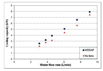
Fig. 9. Tower cooling capacity
