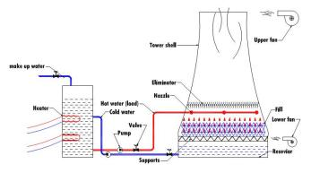
Fig.1 Schematic diagram for experimental test rig [4, and 5].
