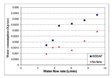
Fig. 8. Water consumed by evaporation.
