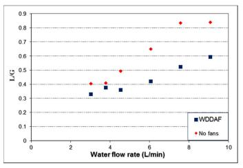
Fig. 5. Water to air mass flow ratio.
